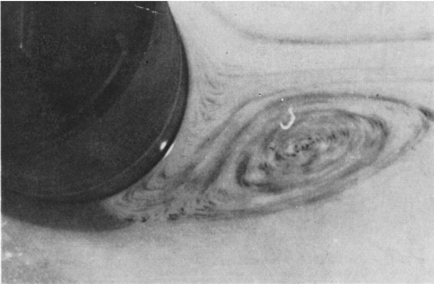
FIGURE 8. Separation over a downstream moving for u_w/\bar{U}_\infty = 0.8 Re = 50 .
